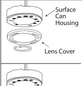
Remove lens cover by twisting counter-clockwise.
